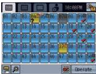
GRID (Zoom Out) Screen Displays the operation status of all groups.
